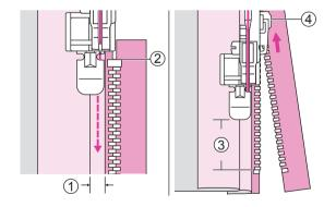
Attach the zipper foot. Attach the right pin for sewing the left side of the zipper. Sew the zipper to the piece of fabric with the extra 3mm, starting from the end of the zipper.
