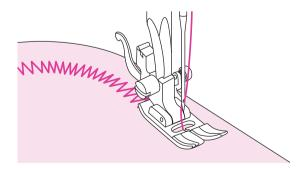
When sewing along a curve while using a zigzag stitch, select a shorter stitch length in order to obtain a finer stitch.
