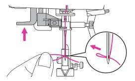
14. Raise the lever straight up, the hook will rotate and pass the thread through the needle eye to form a loop.
