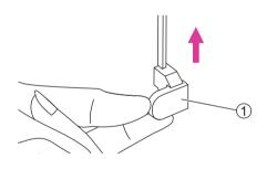
Raise the presser foot lifter and cut the thread. To sew over the same buttonhole, raise the presser foot lifter (it will return to its original position).
