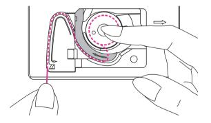
To cut off excessive thread, pull it to the cutter at point (B).
