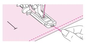
Slightly hold the end of the upper thread and start sewing. Pull two lines together.
