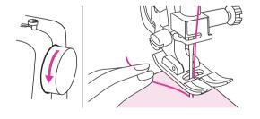
5. Turn the handwheel toward you (counterclockwise) to lower the needle into the fabric at the beginning of the stitching, while holding onto the end of the thread.
