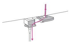
Pass the thread behind the flat, horizontal thread guide through the opening on the right. Then pass the thread through the guide above the needle with the opening on the left. Use the needle threader to thread the needle as described in instructions 10-14.
