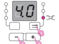
Press the stitch adjustment button, when the tension light is on, the embroidery thread tension can be adjusted.
