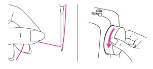
Hold the upper thread with your left hand. Turn the handwheel towards you (counterclockwise) to lower the needle down below the needle plate, continue turning the handwheel to bring the bobbin thread up.
