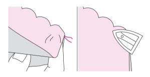
Turn the fabric over and push out the curved seam to the surface and iron it.
