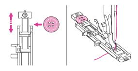
Pull the button holder plate to the back, and place the button in it. Push back the button holder plate against the button to hold it tight.
