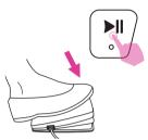
7. Hold the thread tail securely in one hand. Step on the foot control (only in the sewing mode) or long press the start/stop button to start winding the bobbin.
