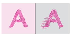
When the upper thread has slack, the thread tension is too loose for embroidering. To increase the tension, press the "+" button.
