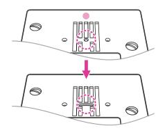
Replacing the straight stitch plate to normal needle plate.
