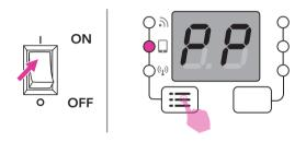
Turn on the power, the screen should show "PP", the middle light on the left should be green and stay on. If it is not, long press the connection mode switch button to change the light.
