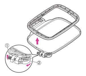
Loosen the fastening screw or open the quick release device (if same type of fabric is used for embroidery).
