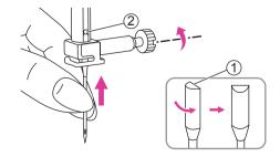
Inserting a proper needle, keep the flat side of the shaft to the back.
