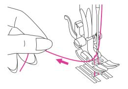
Gently pull on the upper thread to bring the bobbin thread up through the hole in the needle plate. The bobbin thread will come up in a loop.
