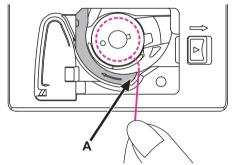
With a finger hold gently on top of the bobbin, please follow the arrow markings and draw the thread into the bobbin thread guide.
