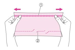
Good for easy to ravel and knit fabrics. It's good for joining durable fabric such as denims.
