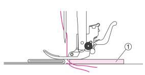
You also can place another piece of fabric with the same thickness at the back of the seam. Or support the presser foot while feeding by hand and sewing toward the folded side.
