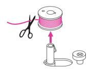
9. Cut the thread and then remove the bobbin from the bobbin winder spindle.
