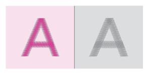
When the bobbin thread is visible on the front of the fabric, the thread tension is too tight for embroidering. To reduce the tension, press the "-" button.
