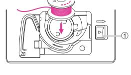
Pull the thread through the slit (A).
