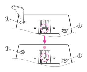
Remove the screws on the needle plate then remove the needle plate.
